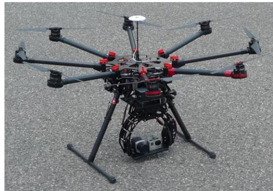
**Figure 1:** The IR Multicopter Drone assembled by the PV LAB at BFH Burgdorf, Switzerland (model S1000 octocopter with camera-system). Photo: BFH-TI.
